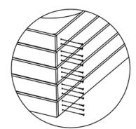
Fix the flat sides together with the help of the screws provided.
