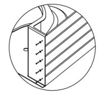
Adjust the flat sides to fit the casing and fix them firmly in place as indicated above using the screws and washers provided.
