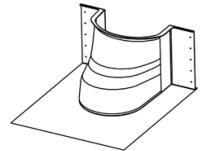
Position the polyethylene casing on the prepared surface.
